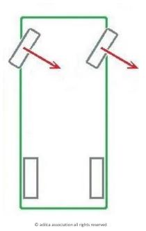
The guiding force originates on the steered wheels upon contact with the ground.
