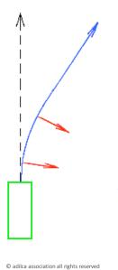
Newton's law: to deflect a mass from its rectilinear path, one must apply a transverse force, represented here by a red arrow.
