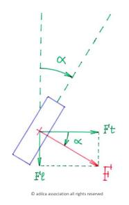
The components of the guiding force F.  $\alpha$ : pivoting angle of the steered wheels. Fr: transverse component. Fr: front-to-back component.
